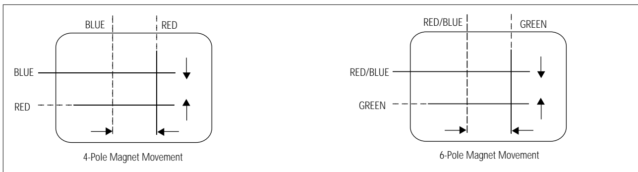
Fig. 4-5 Center Convergence Adjustment
